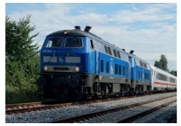
**Prototype**: Railroad Construction and Operating Company Pressnitz Valley Railroad, LLC (PRESS) general-purpose locomotive, road number 218 054-3 (former 218 448-9). Diesel hydraulic locomotive with roof version to accommodate the MTU 12V 956 TB 11 motor. With parallel exhaust hoods and a Behr cooling system in a "V" shape. The locomotive looks as it did from December of 2020.
