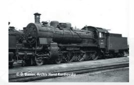
Prototype: Austrian Federal Railways (ÖBB) class 638 passenger locomotive. Former Prussian class P 8. Boiler with 3 domes and without smoke deflectors. Four-axle box-style tender, pilot truck with solid wheels.
