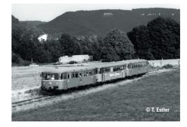
Prototype: German Railroad, Inc. (DB AG) combustion powered rail car (VT), road number 796 702-9, with control car (VS), road number 996 778-7. Dual motor design, built starting in 1955. Used in commuter service (branch lines). The cars look as they did around 1996.
