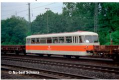
**Prototype**: 2 x type Kkklms 440 without a brakeman's platform and 1 x type VB 98 as a type 395 line inspection car for the German Federal Railroad (DB) around 1989.
