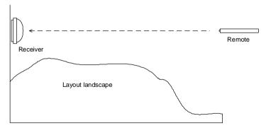
During use, the remote should always be pointed towards the receiver. There is a small red LED placed under the opaque cover of the receiver; this LED illuminates when the receiver "sees" some infrared signal.
