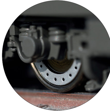
The extremely well executed and modelled disk brakes of the further development are very easy to recognize
