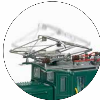
Double-arm pantographs with a wide contact strip
