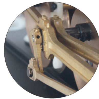
Synchronized with the wheels: Drive rod on the driving wheel
