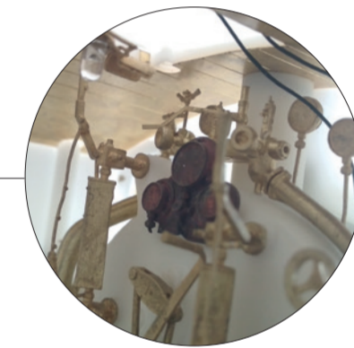
Realized with a high level of detailing: the firebox wall in the cab
